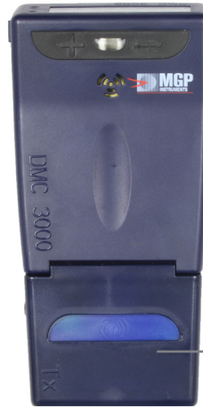
Blue LED for USB Communication
