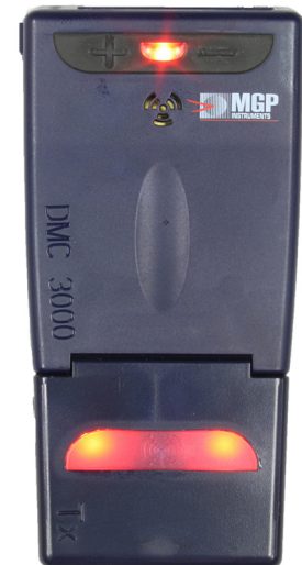
DMC 3000 in Alarm
